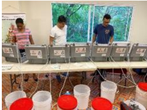
Stream Systems lined up on the tables making chlorine for HCFs in Haiti
